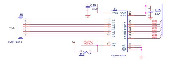
This 8-bit (octal) noninverting bus transceiver contains two separate supply rails; B port has VCCB, which is set at 3.3 V, and A port has VCCA, which is set at 5 V. This allows for translation from a 3.3-V to a 5-V environment, and vice versa.
