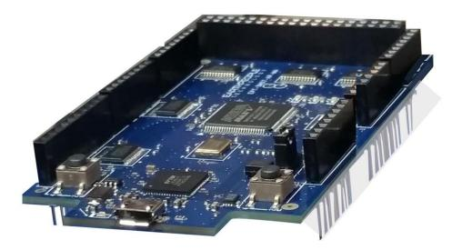
The MegaProLogic is a part of the EPT USB/PLD development system. It provides an innovative method of developing and debugging the users microcontroller code. It can also provide a high speed data transfer mechanism between microcontroller and Host PC.
