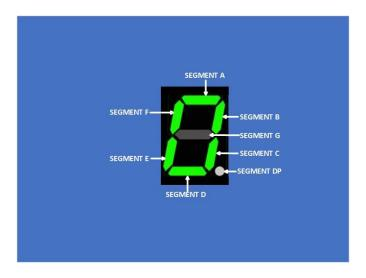
To a pin on the Cyclone 10 FPGA. When the user would like to form a character on the LED Display, the correct segment must be asserted inside the FPGA.
