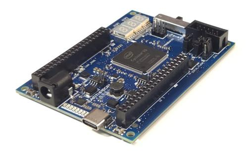
The CycloFlex is an FPGA development board that is designed for the intermediate user with some experience designing FPGA projects.
