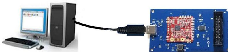
The driver will automatically load. The STATUS LED will light to indicate power has been correctly applied to the SWD Blaster.
