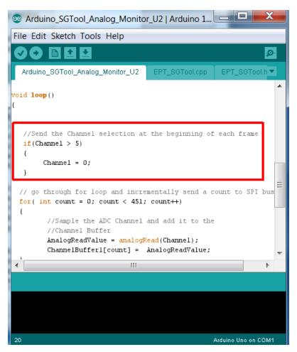
Next, the code enters the buffer loop. A for loop is set up so that one data point is entered into each element of the 500 integer buffer. The channel number was set by the definition of the "Channel" variable.
