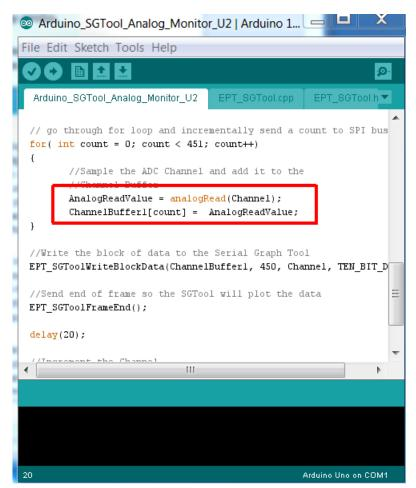
When the for loop has iterated 450 times, the channel buffer has enough data to fill up the Serial Graph Tool display for the selected channel. So, the for loop exits.
