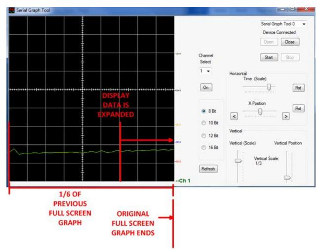
Grab the Horizontal Position Slider and pull it to the left. The display slides to the left. The data is actually being pushed to the right, but the effect is to view older data. Click the "Rst" button to remove the horizontal scaling and display the data without the scale.
