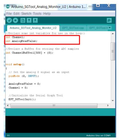
Next, declare the buffer to hold the data that will transmitted to the Serial Graph Tool. The buffer is limited to a size of 500 integers. This limit is important because the Arduino Uno has an SRAM of 2048 bytes. 500 integers will take up half of the memory. The user code will need some amount for the program and some amount for the stack.
