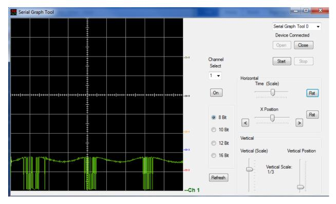
Select Channel 1 and grab the "Time (Scale) " slider and slide it to the left. Notice the signal is zooming out.
