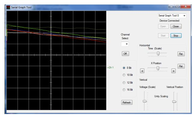
All of the channels will be grouped at the same spot on the graph by default. To separate these channels, click on the drop down box underneath the "Channel Select" lable.
