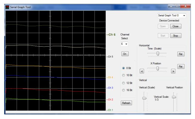
Each channel can also be scaled in the Horizontal Scale. Provide Channel 1 with a signal. A simple way to do this is to touch your finger to the analog input. Then click the "Stop" button. The "Stop" button will cause the Serial Graph Tool to stop filling the circular buffers with new data. All of the previously stored data is preserved in the circular buffers. This allows to you to scroll through the data to view events that occurred in the past.
