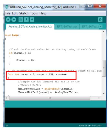
Each time through the for loop, the analogRead() function is called with the Channel number providing the pin number for the analog input. The result of the analogRead () function is stored in the variable AnalogReadValue. This value in turn is stored into the buffer element selected by the for loop.
