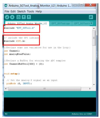
Next, declare an integer Channel and integer AnalogReadValue. The Channel variable will hold the channel number that the data will be written to. The AnalogReadValue will hold the result of the analogRead() function.
