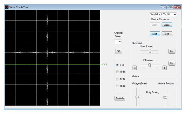
When the Serial Graph Tool connects with the EPT-220X-DB-U2 and the Arduino Uno is running the Analog Monitor code, the display will show all six analog inputs on the screen.
