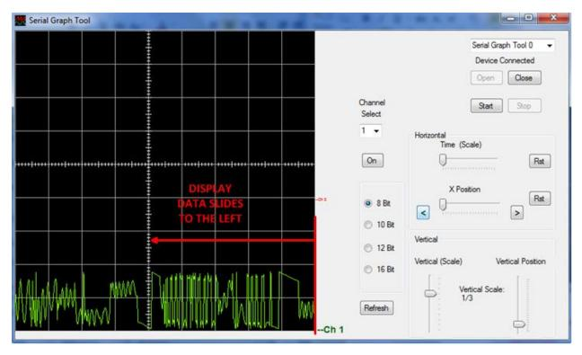
Grab the Horizontal Position Slider and pull it to the right. The display slides to the right. The data is actually being pushed to the left, but the effect is to view the newest data. When the slide right gets to the beginning of the newest data, it cycles around and starts to display the data at the beginning of the circular buffer. This data is the oldest in the buffer, as the newest data overwrites the oldest data in the buffer.
