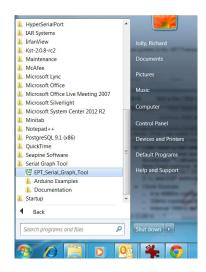
Just click on the Serial Graph Tool icon to launch the application. When the application loads, click on the drop down box at the upper right of the window. Select the Serial Graph Tool 0 in the list. Next, Click "Open" and "Start". The Ardiuno data will display on the graph.
