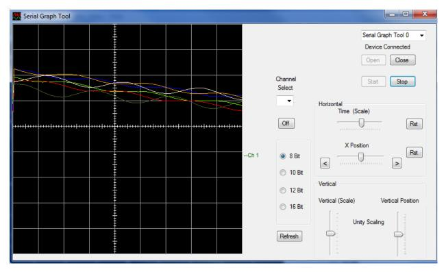
Select a channel and us the "Vertical Position" slider to adjust the position of the channel graph in the display. Notice that the channel indicator highlights in bold when the channel is selected.
