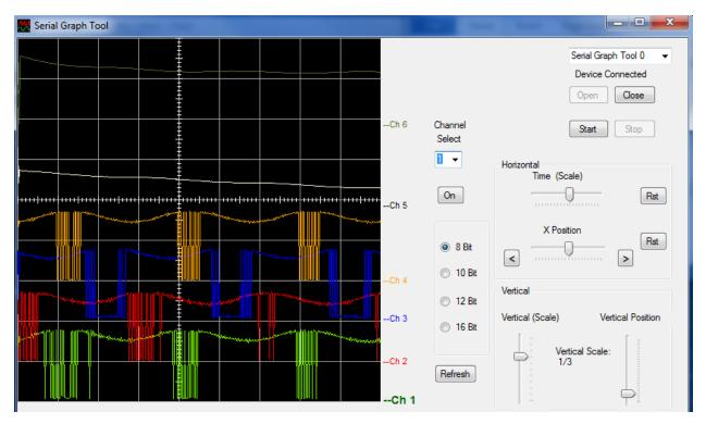
Turn off each channel (except for Channel 1) by first selecting the channel, then clicking on the "On/Off" button directly below the "Channel Select" drop down box.
