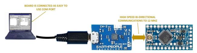
The USB SPI Slave Breakout Board comes with an example C# project that shows the user how completely build a communications project for the external MCU. This project is called the Serial Graph Tool. It comes with an Arduino project that collects analog data and transmits to the PC via the board. The project is completely compiled and working. All source code is provided.
