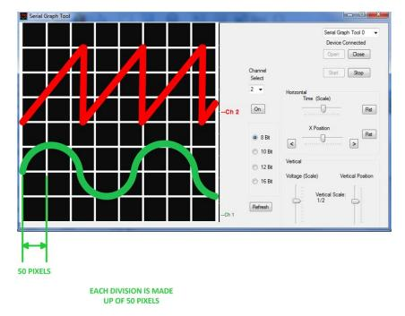
When the Serial Graph Tool receives a FrameEnd command it reads the previous 450 data elements starting from the most recent data element from the selected channel in the circular buffer. It graphs each data element in one pixel. The value of the data element determines the amplitude of the signal.
