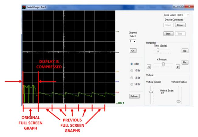
Next, slide the "Time (Scale)' slider all the way to the right. Notice that the display is zooming into the signal.
