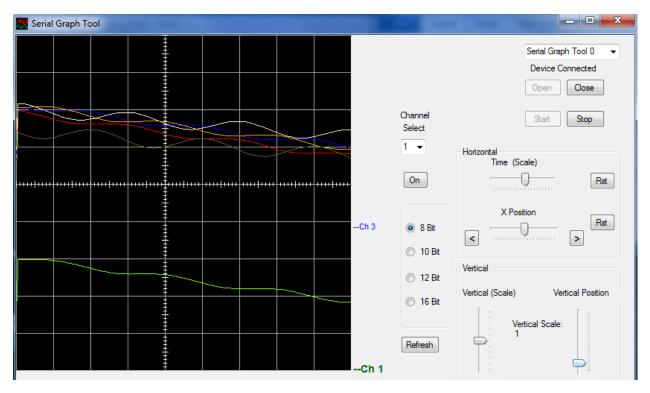
Grab the "Vertical Scale" slider and push up on it until the scale is 1/3. This divides each data element in channel 1 by 1/3.
