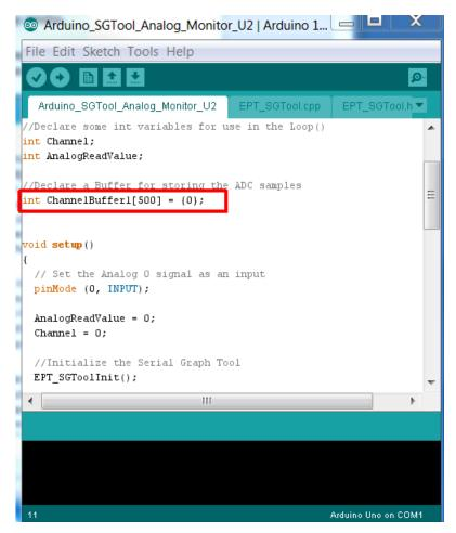
The setup() function is next. The code will set the analog I/O's as inputs, define the variables, and initialize the Serial Graph Tool.
