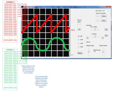
while each pixel is placed on the graph from left to right. The value of all elements in the DataArray can be either 8, 10, 12, or 16 bits. The user will determine which bit selection to use
