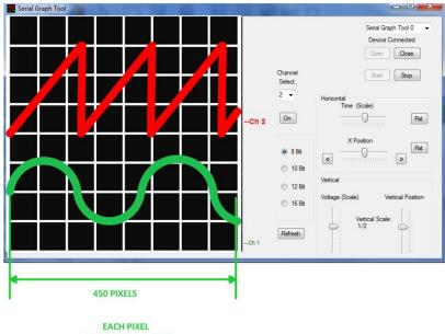
EACH PIXEL CORRESPONDS TO ONE DATA ELEMENT FROM THE SELECTED CHANNEL IN THE CIRCULAR BUFFER
