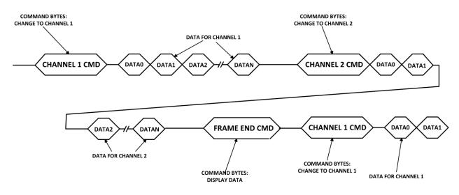
Command. The number of eight bit data packets that follows the "Channel Command" is dependent on user code. There are no restrictions on how many data packets follow the "Channel Command". Each 8 bit data packet in both the commands and data follow the SPI signaling convention. This means the Arduino SPI library is used to send commands and data over the SPI bus.
