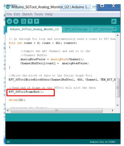
Finally, the "Channel" variable is incremented by one and the process starts over again. This process will go through and record the output for the next analog input (A1) into the "ChannelBuffer1". Then the data is transmitted to the Serial Graph Tool and graphed to the display. This process repeats for all 6 channels. Then, it starts over again at channel zero. This will continue forever, or at least until the power is removed.
