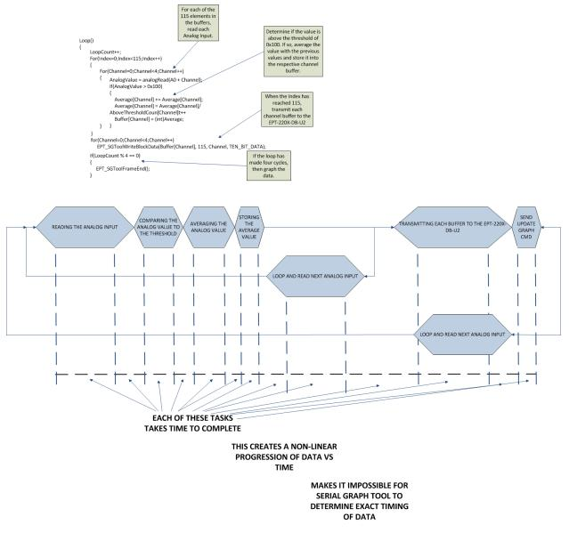
THE USER MUST KEEP UP WITH THE TIMING OF DATA
