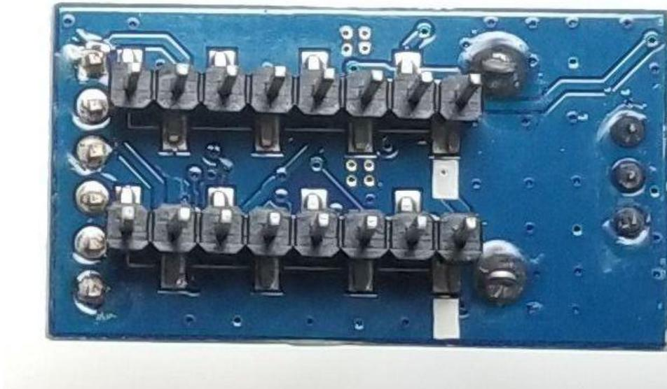
The breadboard headers of the EPT-4901-DA-S1 are surface mounted on the bottom of the board. The board mates perfectly with standard bread boards. The bread board connectors provide the access to the SPI bus. The DAC V<sub>out</sub> is also available on the bread board connectors
