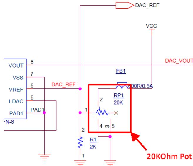
By varying the VREF, the accuracy of the DAC can be improved. This is because the analog output step size between each DAC digital word is reduced. For example, if the VREF is set to 5V, the analog output step size is  $5V/256$  (Digital Steps) = 0.0195V per step. If the VREF is set to 2.5V, the analog output step size is  $2.5V/256$  (Digital Steps) = 0.00976V per step. The smaller the analog step size (or quanta), the more accurate the analog signal can be.
