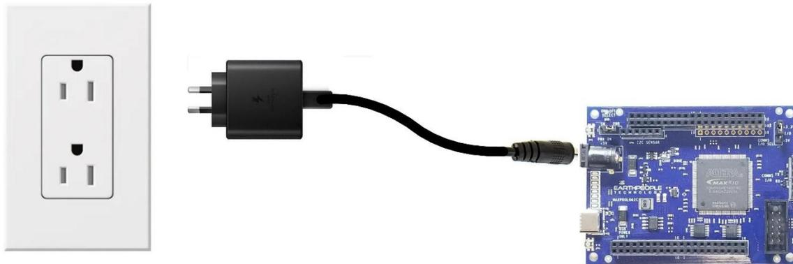
Power the MaxProLogic directly from the wall charger. +5V@2A
