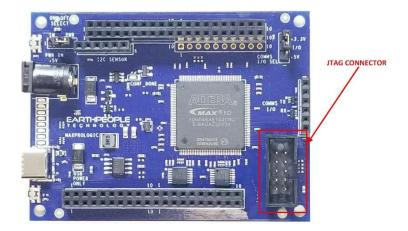
This connector uses the standard Altera Blaster connector pinout.
