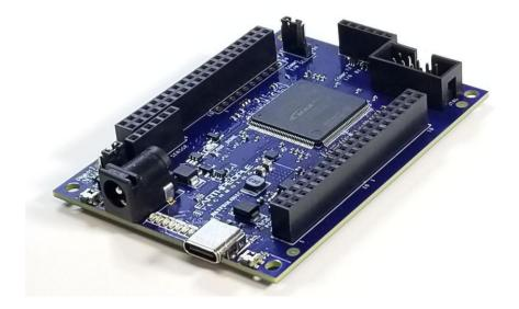
The MaxProLogic is an FPGA development board that is designed to be user friendly and a great introduction into digital design for anyone.
