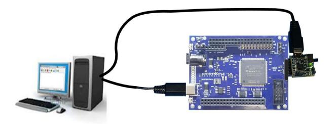
The Communications Connector provides a path between the FTDI Breakout Board and the MAX10 FPGA. It brings both the RX and TX signals into the FPGA at the following pins.
