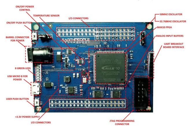
Figure 2 EPT-4CE6-AF Block Diagram
