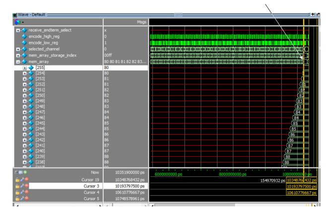
Max\_samples\_reached\_reg is asserted when mem\_array\_storage\_index reaches 0x00ff. The State Machine goes into TRANSFER\_TO\_HOST state.
