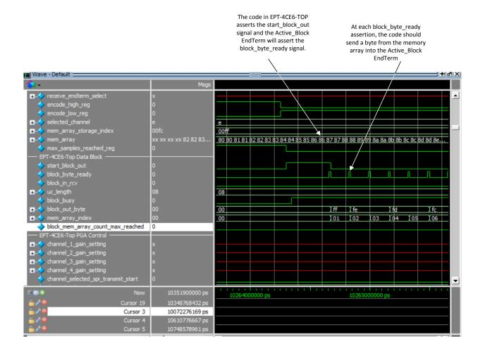
The code continues to increment mem\_array\_index and supply the next byte in the memory array to the Active\_Block EndTerm until block\_mem\_array\_count\_max\_reached asserts. At this point, all the bytes in the memory array have been transferred into the Active\_Block EndTerm. The code in EPT-4CE6-Top returns to idle conditions. The State Machine cycles to HOST\_TRANSFER\_COMPLETE and back to ENCODE\_HIGH. This starts the whole sample, store, and transfer cycle over.
