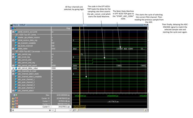
The SPI Communications function in the EPT-4CE6-TOP sends the select channel and gain to the PGA via SPI Bus.
