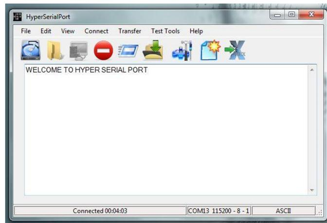
This serial terminal allows you to connect directly with the COM Port that is associated with the Dual Channel FTDI Breakout Board. It's advanced features include the ability to view the characters received as hex values, freeze the screen, record the serial terminal session, and send complete files to the Arduino.
