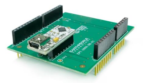
The EPT 201X-DB-U2 is designed to support the UNO board of the Arduino Open source Prototyping Platform. The UNO can communicate as an I2C Master to an I2C Slave device. The EPT 201X-DB-U2 is a USB to Slave I2C device. This will allows users to communicate from the Arduino UNO board to the PC over I2C. Use the Active Host API to quickly and easily create a simulated I2C sensor on the PC. Use the simulated I2C Sensor to debug your Arduino I2C Master communication code.
