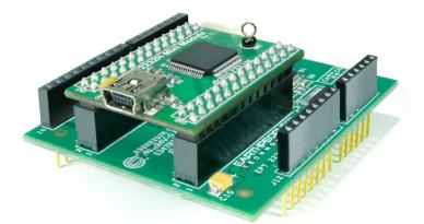
An on board 66 MHz oscillator is used by the EPT Active Transfer Library to provide data transfer rates of 8 Mega Bytes per second. Twenty Four I/O's from the CPLD are attached to three 8 bit transceivers to provide 5 Volt compatible I/O's. These 74LVC245 bidirectional voltage translator/bus transceivers are controlled by one enable and
