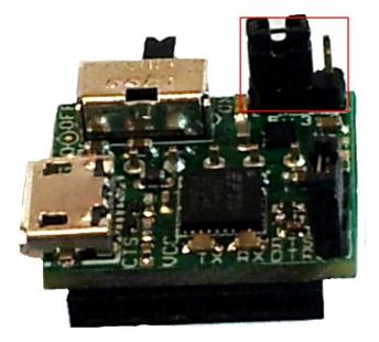
The VisiPort 2 is designed to provide power to the target device. By selecting an interface voltage using the 5V/3V3 jumper, this same voltage will be provided to the user's Arduino. The Visiport 2 has a built in +3.3V power supply and uses the USB power for the +5V. The power provided is:
